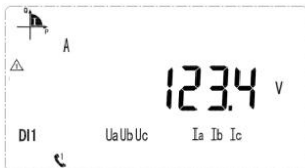
Voltage on A phase is 123.4V
