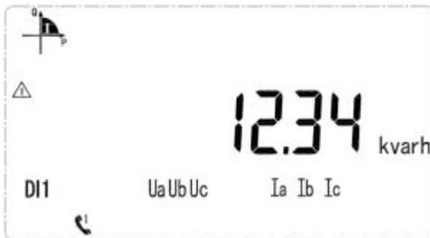
Current forward reactive energy 12.34kWh
