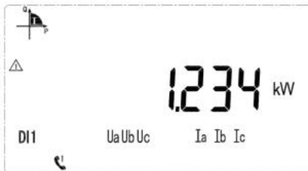
Current total power is 1.234kW
